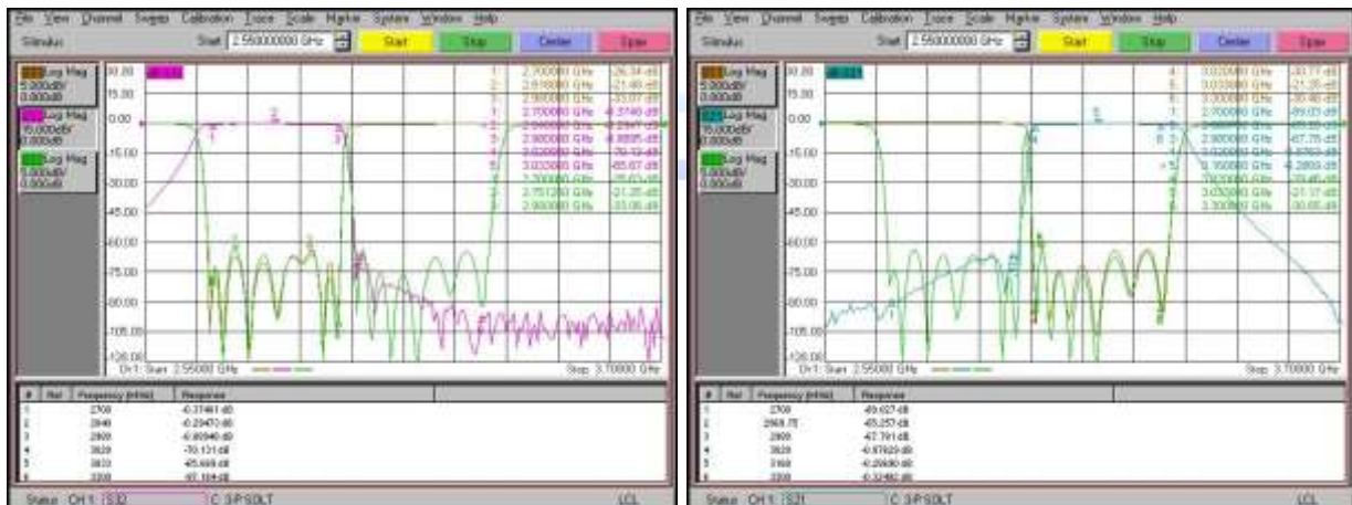
Duplexer Low path Transmission
